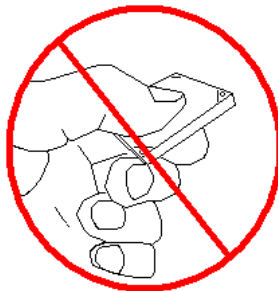
Figure 3. ST1.3 Series improper handling example
